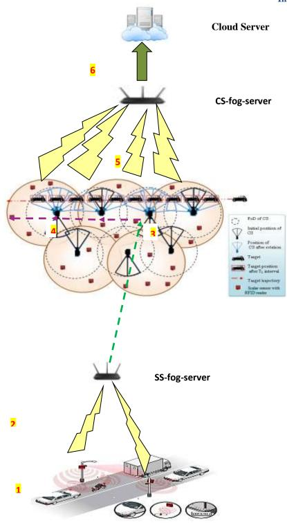
Figure3: Proposed vehicle tracking system model with different activities
